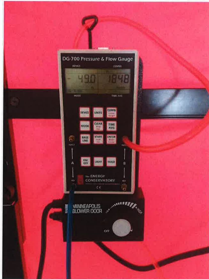
Pic of Blower Door Manometer
