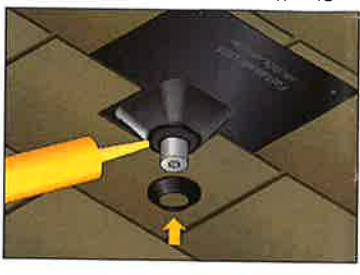
Step 4: Drive lag screw through FastJack base with cordless impact gun until sealed
