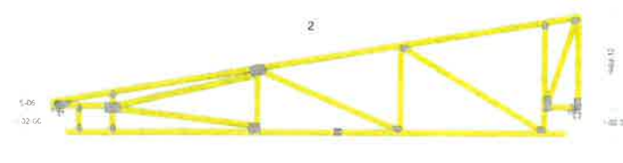
TYPICAL END DETAIL @ GARAGE "RUSS STUBBED BACK 3/4" FOR EDGE OF BLOCK WALL FOR P. WOOD
