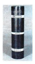
**Product Use:** FLINTLASTIC GTA-FR is designed for use as a roofing membrane cap sheet in APP modified bitumen roof system assemblies over various types of substrates for both new construction and reroofing installations. It is suitable for most low slope roof applications and may be used for roof system flashings including wall treatments, base flashings and field flashings.
