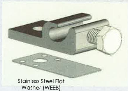
Figure 26. Insert a bolt in the aluminum rail or through the clearance hole in the stainless steel flat washer. Place the stainless steel flat washer on the bolt, oriented so the dimples will contact the aluminum rail. Place the lug portion on the bolt and stainless steel flat washer. Install stainless steel flat washer, lock washer and nut. Tighten the nut until the dimples are completely embedded into the rail and lug. The embedded dimples make a gas-tight mechanical connection and ensure good electrical connection between the aluminum rail and the lug through the WEEB.
