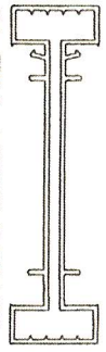
ALL FIN & J FRAMES H-MILLION LARGE VINYL MILLION COVER #VP1-573 EXTRUDED VINYL .071" MIN.
