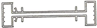
ALL FIN & J FRAMES H-MULLION LARGE VINYL MULLION COVER #VPI-573 EXTRUDED VINYL .071" MIN.
