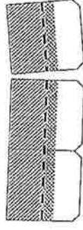
Figure 12-12: Shadow Ridge accessory shingles detach easily from three-piece units to make 72 individual cap pieces.
